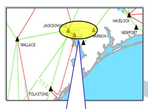
NEW 230 KV TL WITH 6-1590 ACSR OR EQUIVALENT CONDUCTOR. NEW 230 KV SUBSTATION WITH A 200 MVA OR 300 MVA 230/115 KV TRANSFORMER
