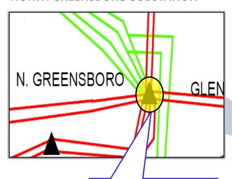
ADD A FOURTH 448 MVA 230/100 KV TRANSFORMER AT NORTH GREENSBORO SUBSTATION
