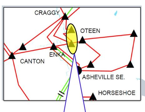
RECONDUCTOR 2.7 MILES OF 115 KV TL WITH 3-795 OR EQUIVALENT. REPLACE 115 KV BREAKERS AND SWITCHES
