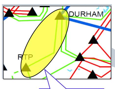
RECONDUCTOR 10 MILES OF 230 KV T.L. WITH 6-1590 ACSR
