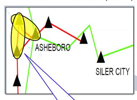
REBUILD 6.5 MILES OF 115 KV TL WITH 3-1590. REPLACE SWITCHES WITH AT LEAST 2000 A CAPABILITY
