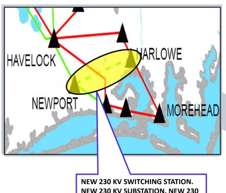
**NEW 230 KV SUBSTATION. NEW 230 KV T.L. WITH 3-1590 ACSR**
