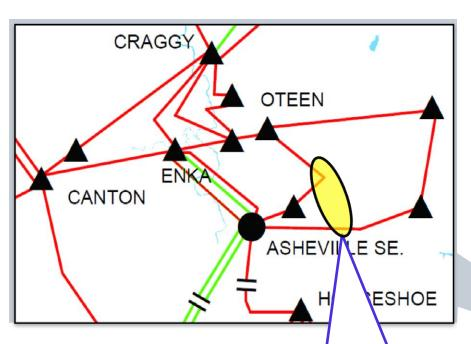
CONSTRUCT 2.2 MILES OF 115 KV TRANSMISSION LINE WITH 795 ACSR. RECONNECT THE BALDWIN 115 KV SUBSTATION.
